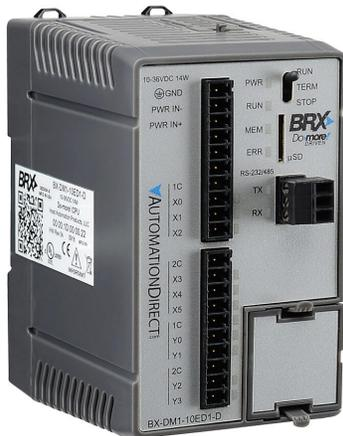
BRX Do-more PLC, 12-24 VDC required, serial port, microSD card slot, Discrete Input: 6-point, AC/DC, Discrete Output: 4-point, sinking.
