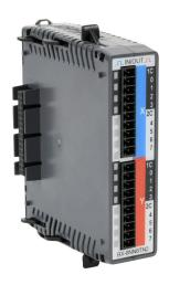
BRX discrete combo module, Input: 8-point, 48 VDC, sinking/sourcing, Output: 8-point, 48 VDC, sourcing, 1A/point. Requires BX-RTB10, BX-RTB10-1 or BX-RTB10-2 terminal block kit or ZIPLink pre-wired cables.
