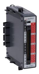
BRX discrete output module, 32-point, 12-24 VDC, sinking, 4 isolated common(s), 8 point(s) per common, 0.5A/point. Requires ZIPLink pre-wired cable.
