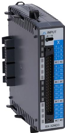
BRX discrete input module, 32-point, 12-24 VDC, sinking/sourcing, 4 isolated common(s), 8 point(s) per common. Requires ZIPLink pre-wired cable.
