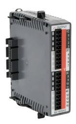
BRX discrete output module, 16-point, 12-24 VDC, sourcing, 4 isolated common(s), 4 point(s) per common, 1A/point. Requires BX-RTB10, BX-RTB10-1 or BX-RTB10-2 terminal block kit or ZIPLink pre-wired cables.
