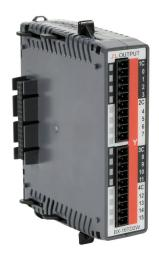
BRX discrete output module, 16-point, 12-24 VDC, sourcing, 4 isolated common(s), 4 point(s) per common, 2A/point, overcurrent, overload and wire-break protection. Requires BX-RTB10, BX-RTB10-1 or BX-RTB10-2 terminal block kit or ZIPLink pre-wired cables.
