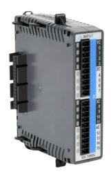
BRX discrete input module, 16-point, 48 VDC, sinking/sourcing, 4 isolated common(s), 4 point(s) per common. Requires BX-RTB10, BX-RTB10-1 or BX-RTB10-2 terminal block kit or ZIPLink pre-wired cables.
