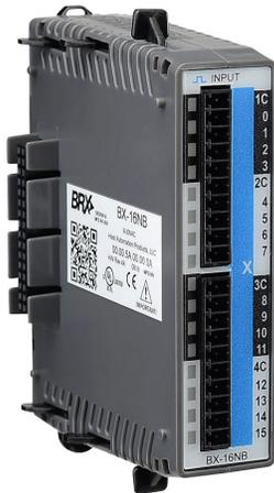
BRX discrete input module, 16-point, 12-24 VAC, 4 isolated common(s), 4 point(s) per common. Requires BX-RTB10, BX-RTB10-1 or BX-RTB10-2 terminal block kit or ZIPLink pre-wired cables.
