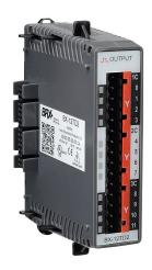
BRX discrete output module, 12-point, 12-24 VDC, sourcing, 3 isolated common(s), 4 point(s) per common, 0.5A/point. Requires BX-RTB08, BX-RTB08-1 or BX-RTB08-2 terminal block kit or ZIPLink pre-wired cables.
