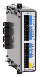
BRX temperature input module, thermocouple, 8-channel, 16-bit resolution, input thermocouple type(s): J, E, K, R, S, T, B, N, C. (1) BX-RTB10 screw terminal block kit included.
