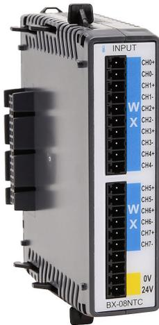
BRX temperature input module, thermistor, 8-channel, 16-bit resolution, input thermistor type(s): 2252, 10K-AN Type 3, 10K-CP Type 2, 5K, 3K and 1.8K ohm. (1) BX-RTB10 screw terminal block kit included.
