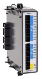
BRX temperature input module, thermistor, 8-channel, 16-bit resolution, input thermistor type(s): 2252, 10K-AN Type 3, 10K-CP Type 2, 5K, 3K and 1.8K ohm. (1) BX-RTB10 screw terminal block kit included.
