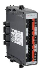
BRX relay output module, 5-point, 12-48 VDC/24-240 VAC, (5) Form C, 5 isolated common(s), 1 point(s) per common, 2A/point. Requires BX-RTB08, BX-RTB08-1 or BX-RTB08-2 terminal block kit or ZIPLink pre-wired cables.
