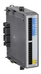
BRX temperature input module, thermocouple, 4-channel, 16-bit resolution, input thermocouple type(s): J, E, K, R, S, T, B, N, C. (1) BX-RTB10 screw terminal block kit included.
