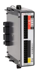
BRX analog output module, 4-channel, current, 16-bit, output current signal range(s) of 0-20 mA and 4-20 mA, external 24 VDC required.
