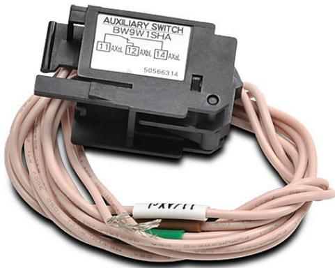
Fuji Electric field installable auxiliary contact, left side mount, SPDT contact(s), 5A @ 125 VAC, 19.69in 20AWG lead wires. For use with Fuji Electric 400A, 630A and 800A frame MCCBs.
