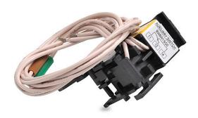
Fuji Electric field installable auxiliary contact, left or right side mount, SPDT contact(s), 5A @ 125 VAC, 19.69in 20AWG lead wires. For use with Fuji Electric 125A and 250A frame MCCBs.
