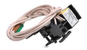
Fuji Electric field installable auxiliary contact, left or right side mount, SPDT contact(s), 5A @ 125 VAC, 19.69in 20AWG lead wires. For use with Fuji Electric 125A and 250A frame MCCBs.
