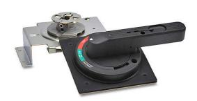
Fuji Electric rotary handle, pistol, black, external front mount, 2-position, lockable in OFF only, defeatable, IP54. For use with Fuji Electric 630A and 800A frame MCCBs. 0.4in shaft and operator included.
