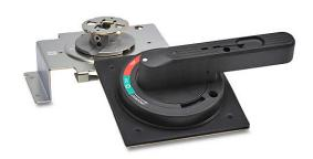
Fuji Electric rotary handle, pistol, black, external front mount, 2-position, lockable in OFF only, defeatable, IP54. For use with Fuji Electric 630A and 800A frame MCCBs. 0.4in shaft and operator included.
