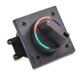
Fuji Electric rotary handle, selector, black, external front mount, 2-position, lockable in OFF only, defeatable, IP54. For use with Fuji Electric 250A frame MCCBs. 0.4in shaft and operator included.
