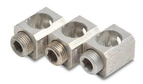
Fuji Electric box type wiring lug, replacement, line or load mount, 1 openings, 2/0 AWG-300 MCM copper only wire(s). Package of 3. For use with Fuji Electric 250A frame MCCBs sizes: 200A, 225A and 250A.
