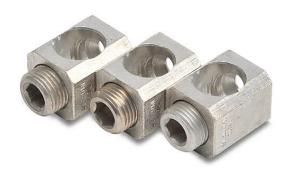
Fuji Electric box type wiring lug, replacement, line or load mount, 1 openings, 2/0 AWG-300 MCM copper only wire(s). Package of 3. For use with Fuji Electric 250A frame MCCBs sizes: 200A, 225A and 250A.
