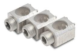
Fuji Electric box type wiring lug, replacement, line or load mount, 1 openings, #1 AWG-3/0 copper only wire(s). Package of 3. For use with Fuji Electric 250A frame MCCBs sizes: 125A, 150A, 160A and 175A.
