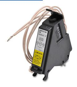
Fuji Electric field installable undervoltage trip, left side mount, 24-48 VAC/VDC sensing range, 19.69in 20AWG lead wires. For use with Fuji Electric 400A, 630A and 800A frame MCCBs.
