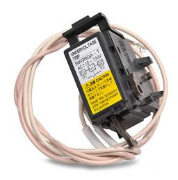
Fuji Electric field installable undervoltage trip, left side mount, 110-130 VAC sensing range, 19.69in 20AWG lead wires. For use with Fuji Electric 125A and 250A frame MCCBs.
