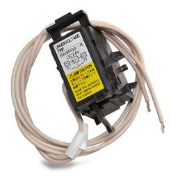
Fuji Electric field installable undervoltage trip, left side mount, 24 VDC sensing range, 19.69in 20AWG lead wires. For use with Fuji Electric 125A and 250A frame MCCBs.
