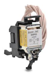
Fuji Electric field installable shunt trip, left or right side mount, 24 VAC/VDC coil voltage, 19.69in 20AWG lead wires. For use with Fuji Electric 125A and 250A frame MCCBs.
