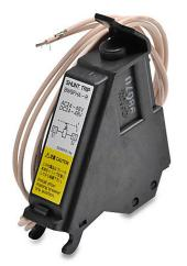
Fuji Electric field installable shunt trip, left side mount, 24-48 VAC/ VDC coil voltage, 19.69in 20AWG lead wires. For use with Fuji Electric 400A, 630A and 800A frame MCCBs.
