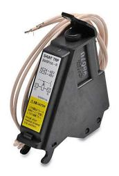
Fuji Electric field installable shunt trip, left side mount, 24-48 VAC/VDC coil voltage, 19.69in 20AWG lead wires. For use with Fuji Electric 400A, 630A and 800A frame MCCBs.
