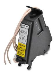
Fuji Electric field installable shunt trip, left side mount, 100-240 VAC/100-220 VDC coil voltage, 19.69in 20AWG lead wires. For use with Fuji Electric 400A, 630A and 800A frame MCCBs.
