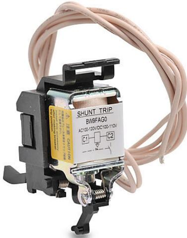
Fuji Electric field installable shunt trip, left or right side mount, 100-120 VAC coil voltage, 19.69in 20AWG lead wires. For use with Fuji Electric 125A and 250A frame MCCBs.
