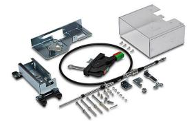
Fuji Electric flange handle, lever, black, external front mount, 2-position, lockable in ON-OFF, defeatable, NEMA 12. For use with Fuji Electric 630A and 800A frame MCCBs. 1.5m cable and MCCB terminal covers included.
