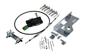
Fuji Electric flange handle, lever, black, external front mount, 2-position, lockable in ON-OFF, defeatable, NEMA 12. For use with Fuji Electric 125A frame MCCBs. 1.5m cable included.
