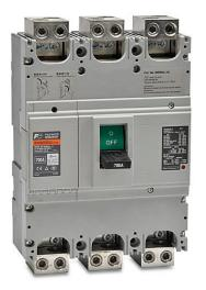
Fuji Electric molded case circuit breaker, 800A frame, 700A, 480 VAC / 250 VDC, 3-pole, characteristics, thermal magnetic, 50kA @ 480 VAC interrupting rating, panel mount. Line and load lug terminals included.
