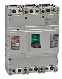
Fuji Electric molded case circuit breaker, 630A frame, 600A, 480 VAC / 250 VDC, 3-pole, characteristics, thermal magnetic, 50kA @ 480 VAC interrupting rating, panel mount. Line and load lug terminals included.
