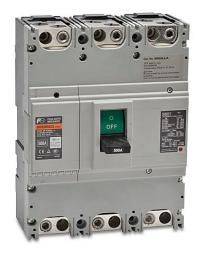
Fuji Electric molded case circuit breaker, 630A frame, 500A, 480 VAC / 250 VDC, 3-pole, characteristics, thermal magnetic, 50kA @ 480 VAC interrupting rating, panel mount. Line and load lug terminals included.
