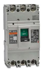
Fuji Electric molded case circuit breaker, 400A frame, 400A, 480 VAC / 250 VDC, 3-pole, characteristics, thermal magnetic, 35kA @ 480 VAC interrupting rating, panel mount. Line and load lug terminals included.
