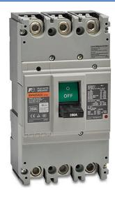
Fuji Electric molded case circuit breaker, 400A frame, 350A, 480 VAC / 250 VDC, 3-pole, characteristics, thermal magnetic, 35kA @ 480 VAC interrupting rating, panel mount. Line and load lug terminals included.
