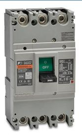
Fuji Electric molded case circuit breaker, 400A frame, 300A, 480 VAC / 250 VDC, 3-pole, characteristics, thermal magnetic, 35kA @ 480 VAC interrupting rating, panel mount. Line and load lug terminals included.
