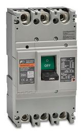
Fuji Electric molded case circuit breaker, 400A frame, 250A, 480 VAC / 250 VDC, 3-pole, characteristics, thermal magnetic, 35kA @ 480 VAC interrupting rating, panel mount. Line and load lug terminals included.
