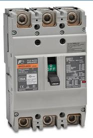
Fuji Electric molded case circuit breaker, 250A frame, 250A, 600 VAC / 250 VDC, 3-pole, characteristics, thermal magnetic, 30kA @ 480 VAC interrupting rating, panel mount. Line and load lug terminals and terminal covers included.
