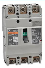
Fuji Electric molded case circuit breaker, 250A frame, 225A, 600 VAC / 250 VDC, 3-pole, characteristics, thermal magnetic, 30kA @ 480 VAC interrupting rating, panel mount. Line and load lug terminals and terminal covers included.
