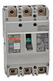
Fuji Electric molded case circuit breaker, 250A frame, 160A, 600 VAC / 250 VDC, 3-pole, characteristics, thermal magnetic, 30kA @ 480 VAC interrupting rating, panel mount. Line and load lug terminals and terminal covers included.
