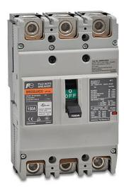
Fuji Electric molded case circuit breaker, 250A frame, 150A, 600 VAC / 250 VDC, 3-pole, characteristics, thermal magnetic, 30kA @ 480 VAC interrupting rating, panel mount. Line and load lug terminals and terminal covers included.
