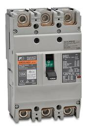
Fuji Electric molded case circuit breaker, 250A frame, 125A, 600 VAC / 250 VDC, 3-pole, characteristics, thermal magnetic, 30kA @ 480 VAC interrupting rating, panel mount. Line and load lug terminals and terminal covers included.
