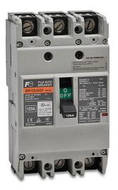
Fuji Electric molded case circuit breaker, 125A frame, 125A, 600 VAC / 250 VDC, 3-pole, characteristics, thermal magnetic, 30kA @ 480 VAC interrupting rating, panel mount. Line and load lug terminals and terminal covers included.
