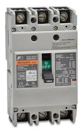
Fuji Electric molded case circuit breaker, 125A frame, 100A, 600 VAC / 250 VDC, 3-pole, characteristics, thermal magnetic, 30kA @ 480 VAC interrupting rating, panel mount. Line and load lug terminals and terminal covers included.
