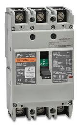
Fuji Electric molded case circuit breaker, 125A frame, 90A, 600 VAC / 250 VDC, 3-pole, characteristics, thermal magnetic, 30kA @ 480 VAC interrupting rating, panel mount. Line and load lug terminals and terminal covers included.
