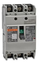
Fuji Electric molded case circuit breaker, 125A frame, 75A, 600 VAC / 250 VDC, 3-pole, characteristics, thermal magnetic, 30kA @ 480 VAC interrupting rating, panel mount. Line and load lug terminals and terminal covers included.
