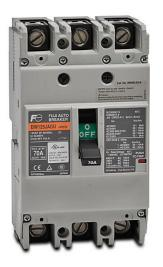
Fuji Electric molded case circuit breaker, 125A frame, 70A, 600 VAC / 250 VDC, 3-pole, characteristics, thermal magnetic, 30kA @ 480 VAC interrupting rating, panel mount. Line and load lug terminals and terminal covers included.
