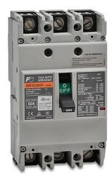
Fuji Electric molded case circuit breaker, 125A frame, 60A, 600 VAC / 250 VDC, 3-pole, characteristics, thermal magnetic, 30kA @ 480 VAC interrupting rating, panel mount. Line and load lug terminals and terminal covers included.
