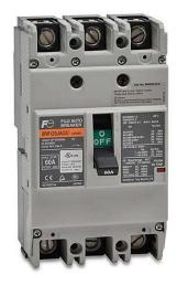
Fuji Electric molded case circuit breaker, 125A frame, 60A, 600 VAC / 250 VDC, 3-pole, characteristics, thermal magnetic, 30kA @ 480 VAC interrupting rating, panel mount. Line and load lug terminals and terminal covers included.
