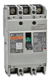
Fuji Electric molded case circuit breaker, 125A frame, 50A, 600 VAC / 250 VDC, 3-pole, characteristics, thermal magnetic, 30kA @ 480 VAC interrupting rating, panel mount. Line and load lug terminals and terminal covers included.
