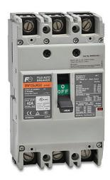
Fuji Electric molded case circuit breaker, 125A frame, 40A, 600 VAC / 250 VDC, 3-pole, characteristics, thermal magnetic, 30kA @ 480 VAC interrupting rating, panel mount. Line and load lug terminals and terminal covers included.
