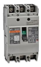
Fuji Electric molded case circuit breaker, 125A frame, 30A, 600 VAC / 250 VDC, 3-pole, characteristics, thermal magnetic, 30kA @ 480 VAC interrupting rating, panel mount. Line and load lug terminals and terminal covers included.
